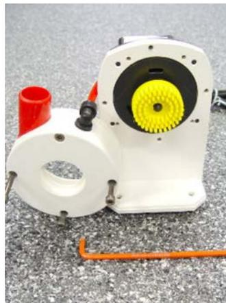
If the impeller group extremely calcified, solve the plate between engine and rotor. Cover enter with a small slot screwdriver, **!carefully!**
