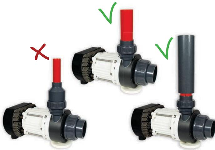
If there is a danger that the pressure pipe gets completely blocked (e.g. by a ball valve) a bypass has to be installed in the pressure pipe, so that **always** a minimal flow of water through the pump is guaranteed.
