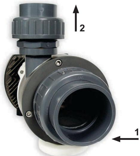
It has to be assured that the pump can be de-aerated through the outlet (2). The pump should ideally be placed beneath the water level.
