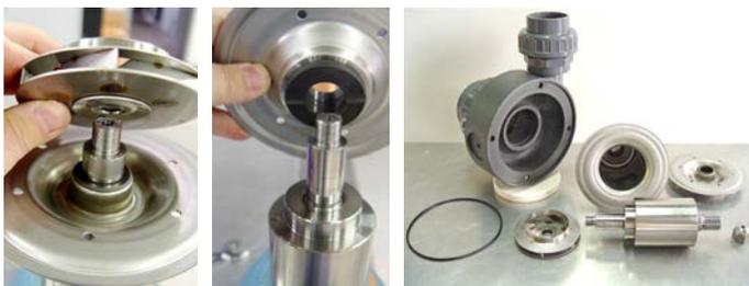
Decalcify all individual parts after disassembly of all component parts.
