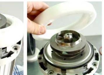
Use a large flat screw driver to carefully lift off the flange ring and remove it.
