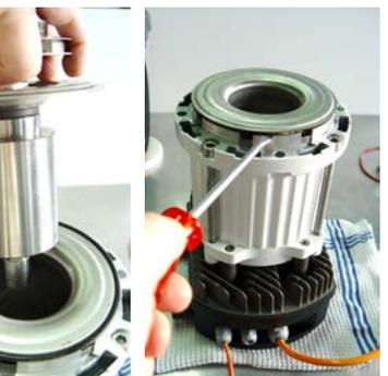
Grasp the impeller unit and pull it out.
