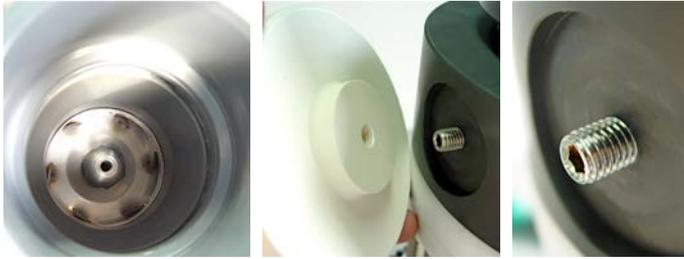
Check the impeller for freedom of movement. Unscrew the pump base and the V4A grub screw from the pump head.
