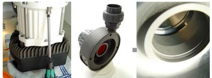
**Assembly of pump head:** Always ensure that the solid pump head does not rest sideways on the suction ring of the impeller. Therefore, it is recommended to fasten the pump head in the inlet duct from the top and then tighten the 4 M10 housing screws slightly cross-wise.
