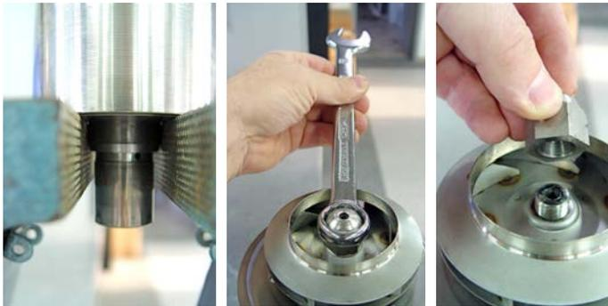
When unscrewing the impeller, clamp the unit in a vice.
