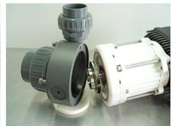
Use Allen wrench M8 to turn off the 4 housing screws and remove the head.
