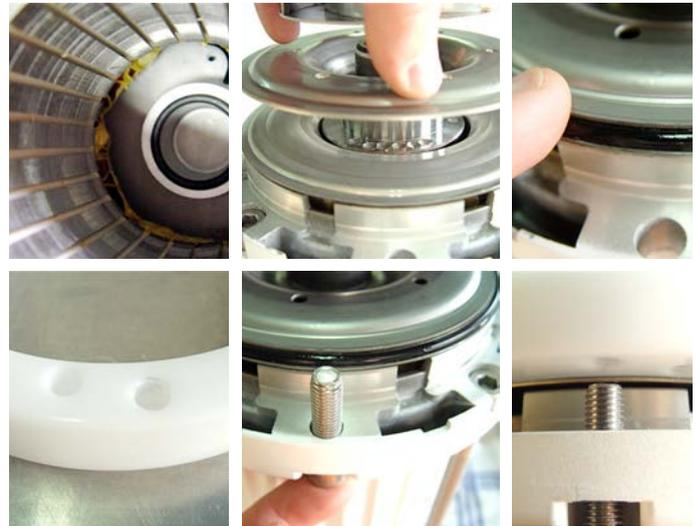
**Assembly:** Fasten the O-ring in the groove in the stator space. Insert containment shell and impeller to the stop. Install and grease the O-ring.
