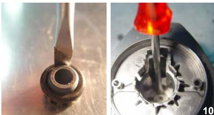
If the bearing is mounted into the appropriate notch, the O-ring must be firmly pressed into the notch using a medium-size slotted screwdriver (fig. 10).
