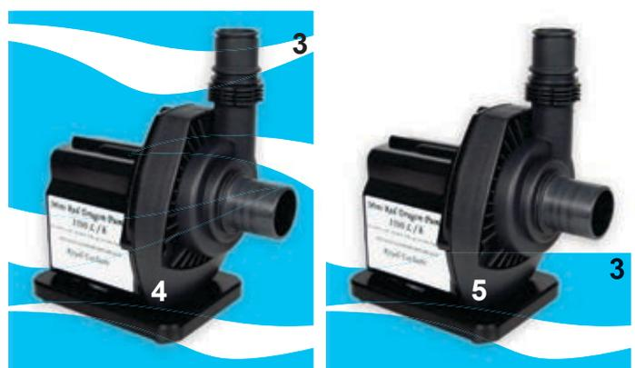
The pump can be placed submersed (4) or out of the water (dry) (5). In the case of a dry placement, adequate air ventilation has to be assured. Furthermore the pump may not be exposed to direct sunlight. Place the pump as close as possible to the actual water connection; hence the inlet piping has to be as short as possible.
