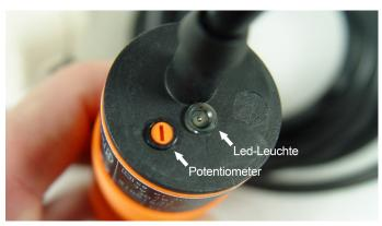
The switching distance can be adjusted at the potentiometer with the help of the screwdriver remote with.
