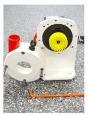
If the impeller group extremely calcified, solve the plate between engine and rotor. Cover enter with a small slot screwdriver, !carefully!
