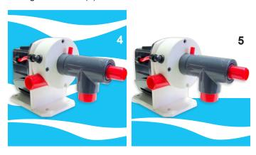
The pump can be placed submersed (4) or out of the water (*dry*) (5). In the case of a dry placement, adequate air ventilation has to be assured. Furthermore the pump may not be exposed to direct sunlight. Place the pump as close as possible to the actual water connection; hence the inlet piping has to be as short as possible.
