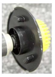
If the bearing fits on the shaft, like shown on the picture on the left, when pulled out, then manually remove it from the shaft. And the bearing after removal from the shaft. (shown on the picture on the right)
