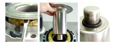
*Caution:* The stator is located just behind the flange. Please note that the coil must not be touched or damaged. Remove the containment shell.
