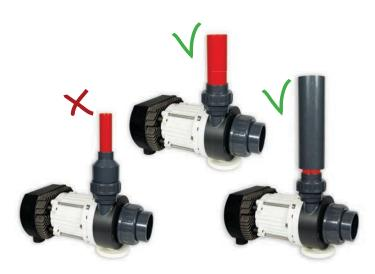
If there is a danger that the pressure pipe gets completely blocked (e.g. by a ball valve) a bypass has to be installed in the pressure pipe, so that **always** a minimal flow of water trough the pump is guaranteed.
