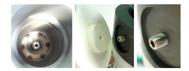
Check the impeller for freedom of movement. Unscrew the pump base and the V4A grub screw from the pump head.
