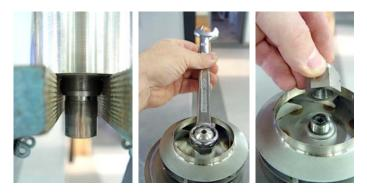
When unscrewing the impeller, clamp the unit in a vice. *Caution:* Never clamp the axis to the slide bearing!! Clamp only at the upper shaft area as shown in the picture. Use an M24 wrench to loosen the cap nut clockwise (left-hand thread) and disassemble the impeller and bearing plate.
