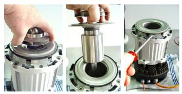
Grasp the impeller unit and pull it out. In case of extreme blocks, pour the decalcifier into the solenoid armature space through 6 mm holes and leave approx. 20 minutes. Then carefully lift off the containment shell using a large screw driver.
