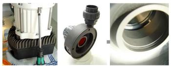
**Assembly of pump head:** Always ensure that the solid pump head does not rest sideways on the suction ring of the impeller. Therefore, it is recommended to fasten the pump head in the inlet duct from the top and then tighten the 4 M10 housing screws slightly cross-wise.
