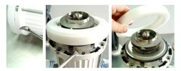
Use a large flat screw driver to carefully lift off the flange ring and remove it.
