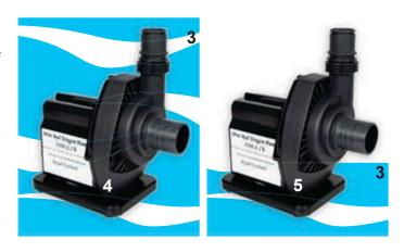
The pump can be placed submersed (4) or out of the water (*dry*) (5). In the case of a dry placement, adequate air ventilation has to be assured. Furthermore the pump may not be exposed to direct sunlight. Place the pump as close as possible to the actual water connection; hence the inlet piping has to be as short as possible.
