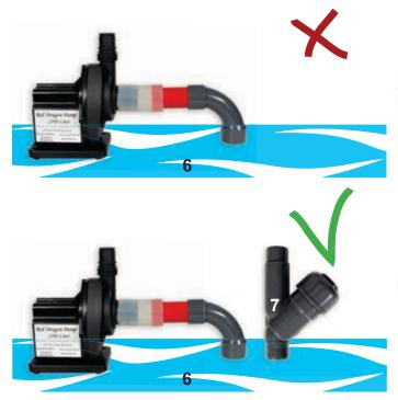
If the pump is placed above the water level (6) the installation of a backpressure valve (7) is mandatory. In this case the inlet piping of the pump has to be filled with water before the pump is set to operation. In such a setup the risk of the pump to run dry is very high, when the back pressure valve does not work properly. Damages which are caused by the pump running dry are excluded from warranty.
