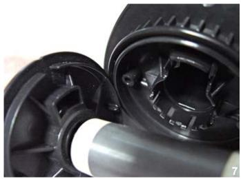
**6.1 Descaling and cleaning the impeller**Now descale the impeller unit using a suitable deliming bath. **Never** use **hydrochloric acid** - **not even diluted!**
