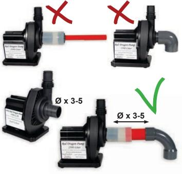
If the inlet piping is longer than max.  $\emptyset$  x 10 the inlet piping has to be 1 or 2 sizes larger than the intake of the pump.
