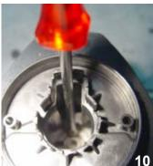
If the bearing is mounted into the appropriate notch, the Oring must be firmly pressed into the notch using a medium-size slotted screwdriver (*fig.* **10**).
