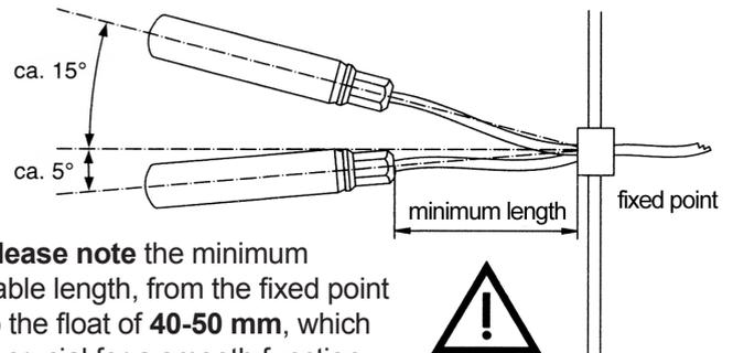
**Please note** the minimum cable length, from the fixed point to the float of **40-50 mm**, which is crucial for a smooth function.
